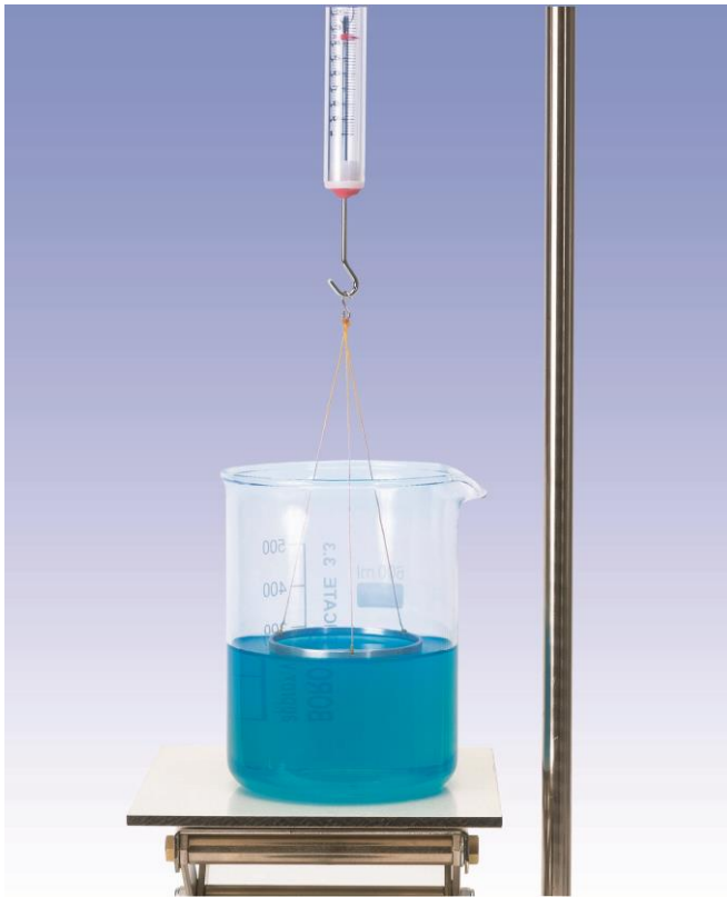
Fig. 3: Experiment set-up for surface tension measurements
